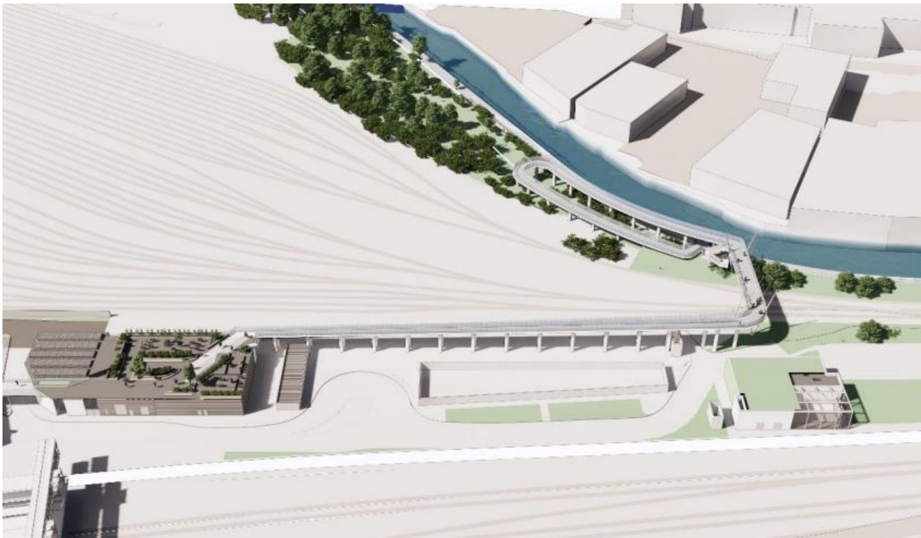
Image of Mott McDonald Option 2a for an 'elevated ped/cycle' connection from Grand Union Canal southern towpath to OOC station at upper level. Does not show staircase from Mitre bridge to towpath (next slide).
