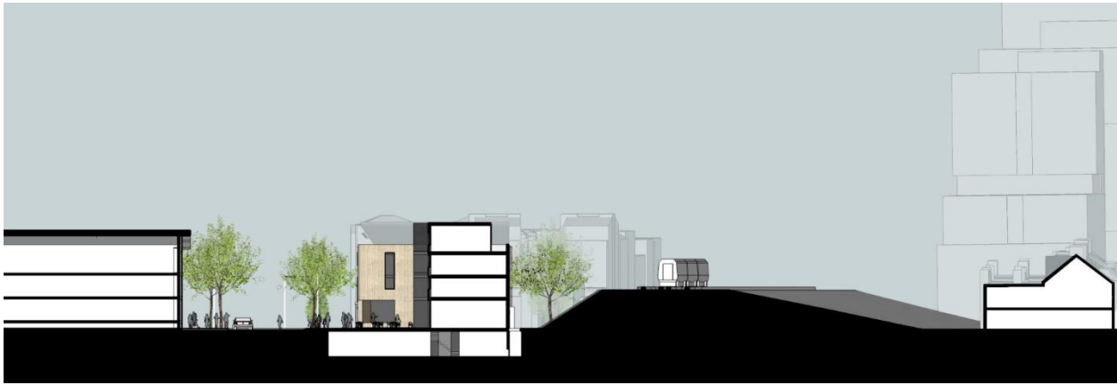
Section through Latimer Road, railway line (Borough boundary) and Eynham Road showing height levels assuming redevelopment of Units 1-14 under StQW Draft Policies. Building shown on the eastern side of Latimer Road (to left of image) is the existing mixed use development at Nos 290-294.
